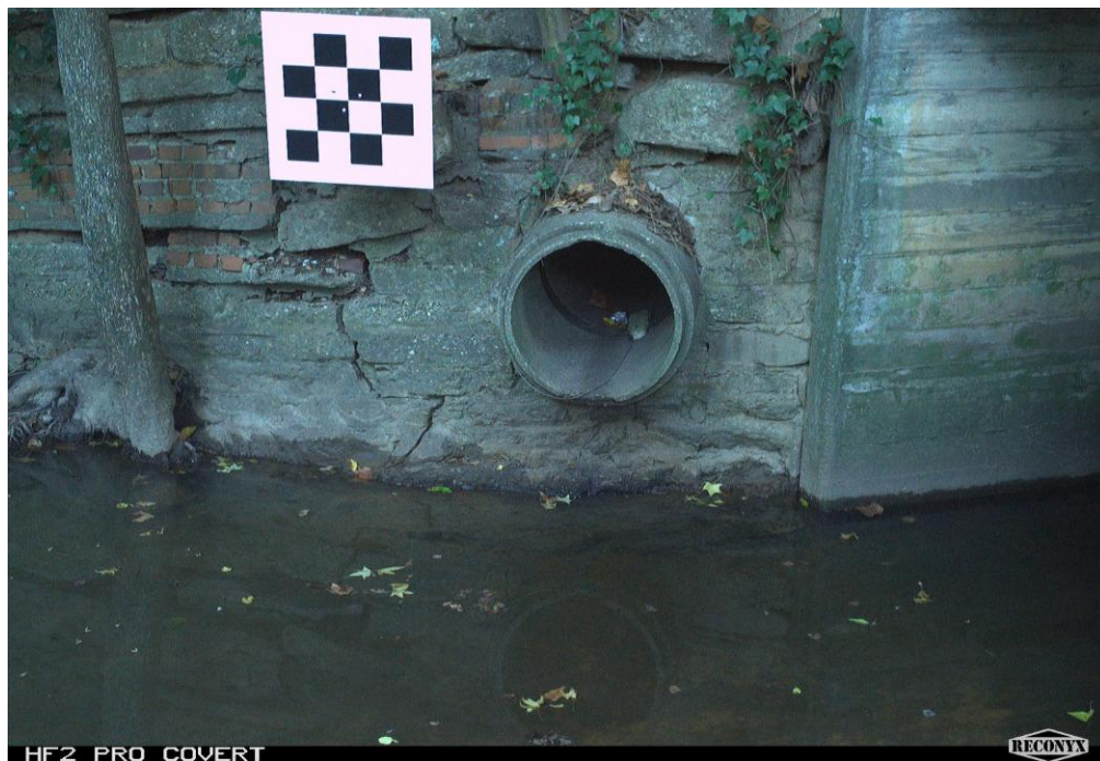
Figure 5: Calibration setup with reference object (chessboard pattern) embedded and aligned with the stormwater outlet
