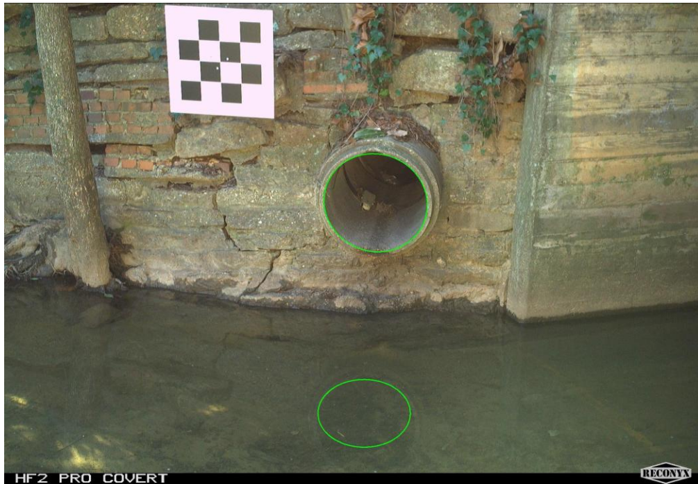
Figure 4: An example of a false positive detection: the Mask R-CNN model identifies both a culvert and its reflection in a pond.
